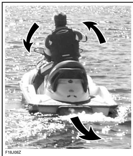
TYPICAL - STEERING DIRECTION REVERSED WHEN BACKING
