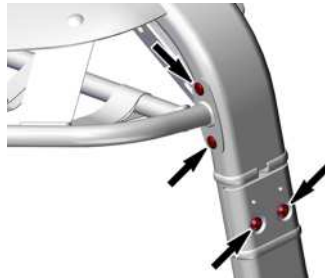
FRONT BIMINI STRUCTURE SCREWS – LH SIDE
