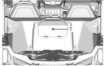
1. Coolant tank access cover
