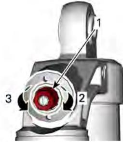
**SMORZAMENTO IN COMPRESSIONE AD ALTE VELOCITÀ (UTILIZZARE UNA CHIAVE INGLESE DA 17 MM)**
