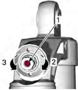
**SMORZAMENTO IN COMPRESSIONE A BASSA VELOCITÀ (UTILIZZARE UN CACCIAVITE)**
