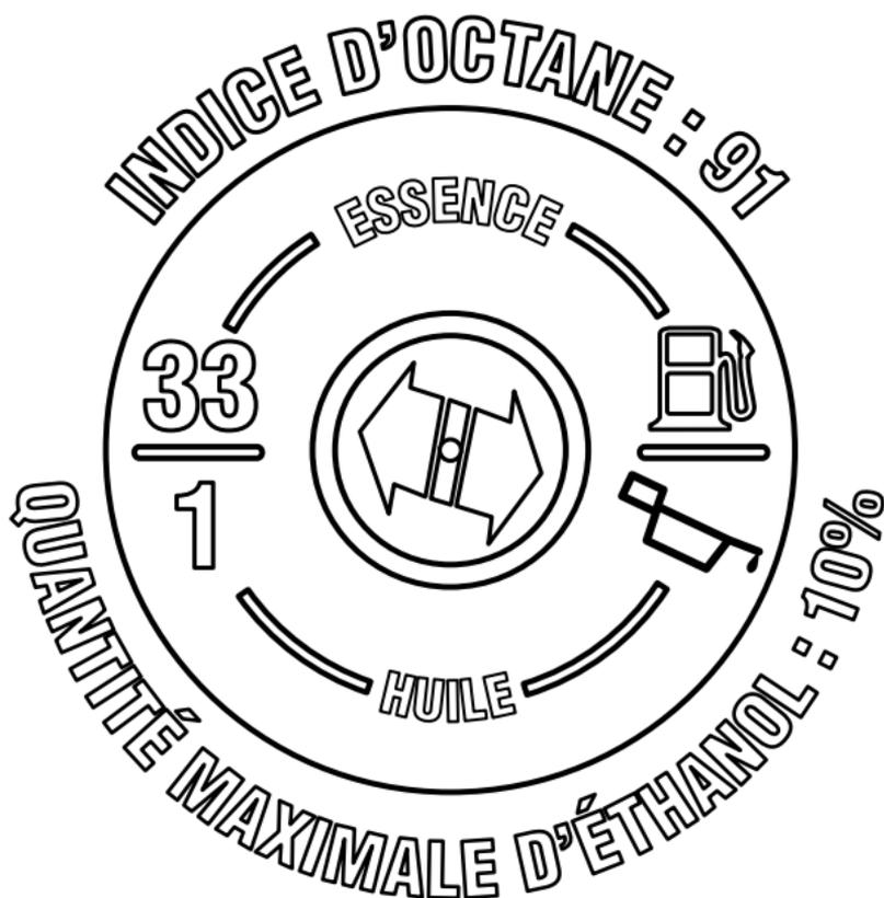
**SUR LE BOUCHON DU RÉSERVOIR DE CARBURANT (DANS
