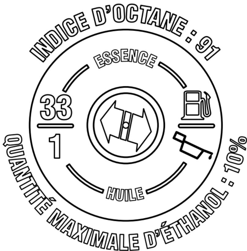
**SUR LE BOUCHON DU RÉSERVOIR DE CARBURANT (DANS LES PAYS UTILISANT DES INDICES D'OCTANE AKI (RON + MON)/2 AFFICHÉS À LA POMPE)**
