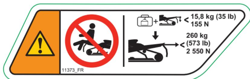
**CHARGE CARGO MAXIMALE ET CAPACITÉ DE REMORQUAGE - ÉTIQUETTE D'AVERTISSEMENT**
