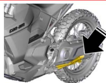
If vehicle is tipped over, lift up by grabbing handlebar and rear seat structure.
