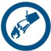
UTILISER UNE GRANDE QUANTITÉ D'EAU POUR ÉTEINDRE LE BLOC-BATTERIE HAUTE TENSION
