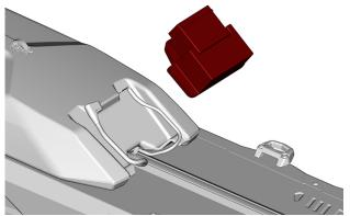
Install the battery hold down bracket. Secure with the previously removed screw and flat washer.
