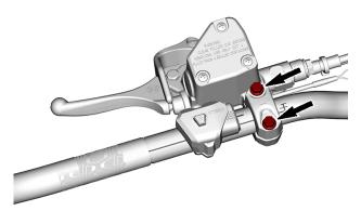
Locate the reference mark on the handlebar and respect the distance and rotation limits.
