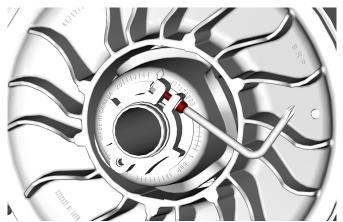
Using the suspension adjustment tool provided in the tool kit, turn the adjustment ring 1/4 turn at a time then rotate the driven pulley to properly set the belt between the pulley sheaves.
