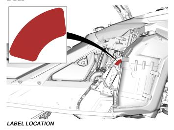
Factory Installed Chain and Sprockets - Notice Label Turbo R Engine
