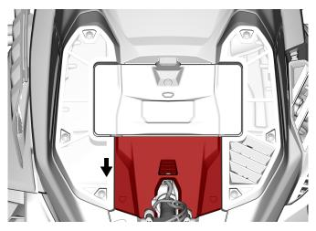
Check coolant level at room temperature. Liquid should touch the flat surface of the eyesight.
