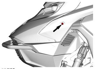
LH SIDE5. Loosen the air intake duct clamp.
