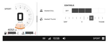
**NOTE**: The heated grips ratio can only be adjusted using the touchscreen. The touchscreen is not available when riding.
