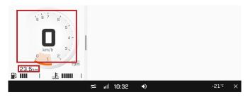
In full gauge view, long press the lower center of the screen to show one the following information. Cycle through the informations with additional long presses.
