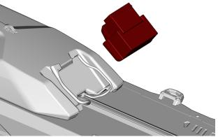
6. Remove the battery from the battery support.
