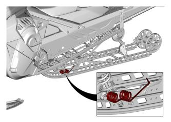
Ice scratchers must be used whenever the vehicle is operated on a trail, hard snow or ice.
