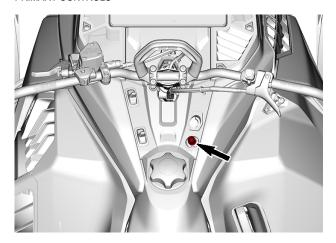
The engine cut-off switch (tether cord) is located on the console.
