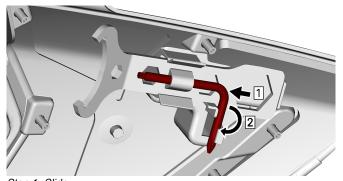
Step 1. Slide Step 2. Rotate and clip
