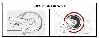
From factory, the adjustable stopper strap is set in the way where the "AGILE" position = setting #4 on regular stopper strap. The "PRECISION+" position = setting #7 on the regular stopper strap.
