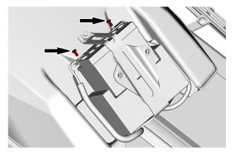
4. Remove the battery hold down bracket.
