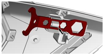
Slide the pulley expander and headlight adjustment tool long end into hole.
