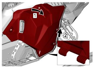
Step 1. Pivot side panel Step 2. Slide side panel
