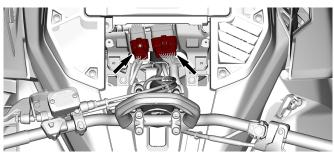
6. Install the access cover by sliding it forward.
