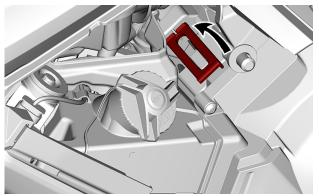
Release the pulley guard safety lock and slide the panel outwards.
