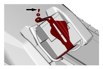
5. Remove the battery with the battery support.
