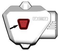
Apply throttle slowly and evenly. Allow drive pulley to engage then accelerate carefully.
