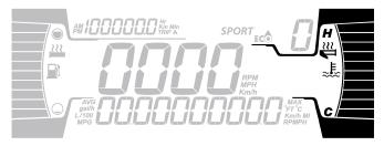
Heated grips and throttle lever will be OFF when there are no bars displayed on the gauge.
