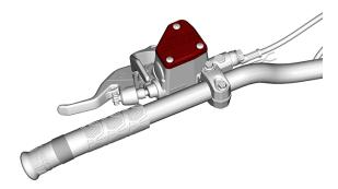
2. Remove the screws retaining the reservoir cap.
