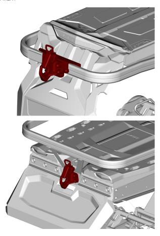
To open the hook, push and turn the handle to retract locking plate.
