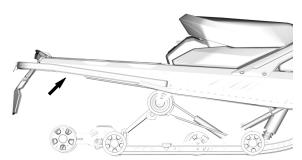
5. Pull on the oil pump cable - at the adjustment - until the exhaust gas turns to darker smoke.
