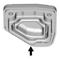
6. Reinstall reservoir cap and screws. Tighten to specification.
