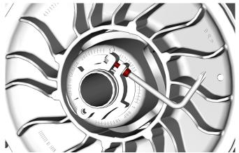
5. Using the suspension adjustment tool provided in the tool kit, turn the adjustment ring 1/4 turn at a time then rotate the driven pulley to properly set the belt between the pulley sheaves.
