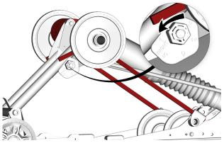
SPRING PRELOAD ADJUSTMENT RH — TYPICAL
