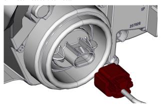
9. Unlock bulb by turning it counterclockwise. 10. Pull bulb out.
