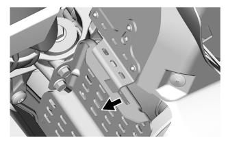
Position the rear portion of the belt guard over the retainer and secure it using the retaining pin.
