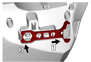
Slide the Pulley expander and headlight adjustment tool short end into hole.
