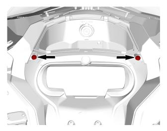
4. Lift the front of the gauge support, then slide it forward to remove it.
