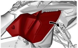
3. Slide the panel hinge off the bottom pan.
