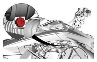
10. Remove the upper body module retaining screws on both sides.
