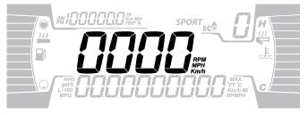
Display the RPM of the engine or the vehicle speed in Km/h or MPH.
