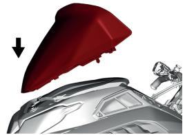
Lower the windshield until both side pins are in their rubber grommets.
