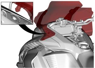
Grasp the windshield assembly under the sides of the windshield support. Lift both sides of the windshield assembly until the side anchor posts are clear of their sockets.
