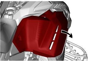
3. Slide the panel hinge off the bottom pan.
