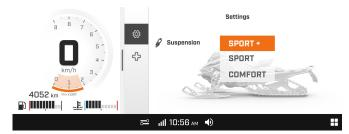
Changing the Smart-Shox mode using the center gauge 3. Select the suspension as the center gauge.
