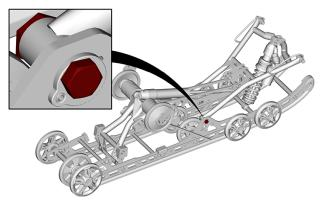
6. Remove the cam, pivot 180°, reinstall in the rail.
