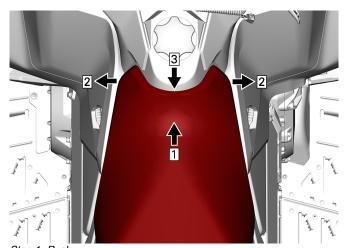
Step 1. Push Step 2. Pull Step 3. Slide backward With Heated Seat
