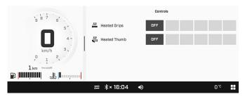
The heated grips and throttle lever heat levels can be adjusted to de desired intensity.
