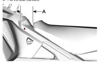
A = Just enough to disengage the seat from the fuel tank 4. Disconnect the heated seat harness.
