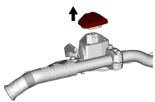
Add fluid as required. Do not overfill. Use only the recommended brake fluid.
