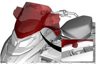
Grasp the windshield support by the front of the assembly. Lift the front anchor post from its socket and remove the windshield assembly.
