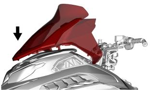
Lower both sides of the windshield assembly until the side anchor posts are secured into their sockets.
