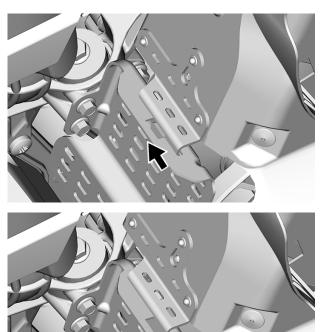
3. Insert belt guard tab between bottom pan and hook.
