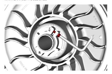
Using the suspension adjustment tool provided, turn the ring 1/4 turn at a time then rotate the driven pulley to properly set the drive belt between the pulley sheaves.
