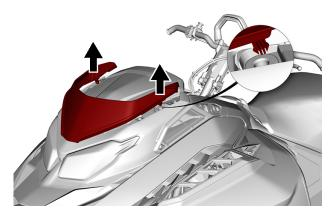
3. Disengage the center pin and remove the windshield assembly.
