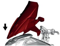
Lower the windshield assembly until the anchor posts are seated in their sockets.
