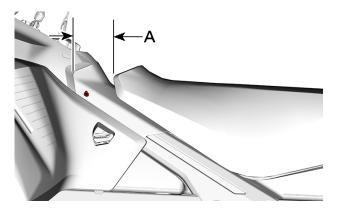
A = Just enough to connect the heated seat harness With Heated Seat
