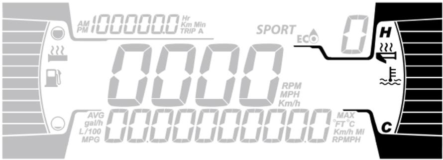
Heated grips and throttle lever will be OFF when there are no bars displayed on the gauge.
