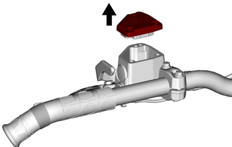
4. Add fluid as required. Do not overfill. Use only the recommended brake fluid.
