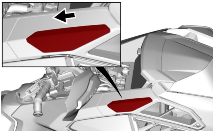
5. If equipped, remove the windshield with side deflectors.
