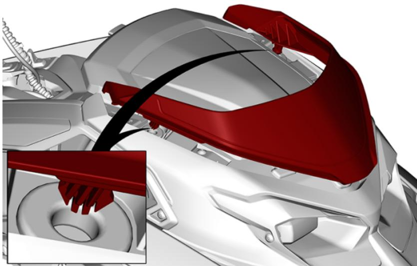
3. Disengage the center pin.
