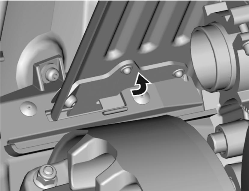
3. Position rear portion of the drive belt guard over the retainer and secure it using the retaining pin.
