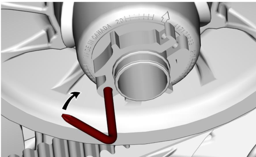
4. Open the driven pulley by screwing the tool in.
