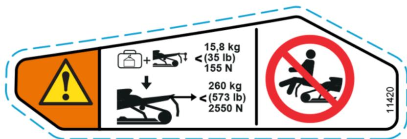
**MAXIMUM CARGO LOAD AND TOWING CAPACITY —
