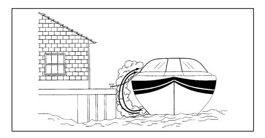
Be sure to provide adequate ventilation. If the windshield has vents, open them before getting underway to increase positive air flow and decrease the chances of CO accumulation.
