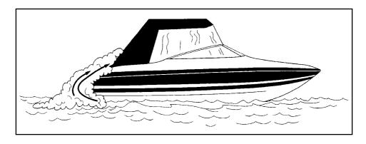
Even with the best boat design and construction, CO may still accumulate in enclosed or confined areas under certain conditions. Continually observe passengers for symptoms of CO poisoning.
