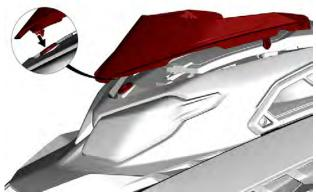
Lower the rear of the windshield assembly and insert the side anchor posts into their sockets. Press down until the posts click into place.
