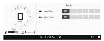
The heated grips and throttle lever heat levels can be adjusted to de desired intensity.
