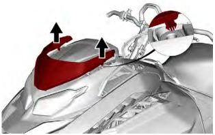
Grasp the windshield support through the vent slot in the front of the assembly. Lift the windshield assembly to clear the front anchor post from its socket. Remove the windshield assembly.
