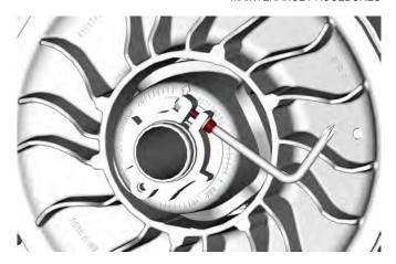
2. Using the suspension adjustment tool provided, turn the ring 1/4 turn at a time then rotate the driven pulley to properly set the drive belt between the pulley sheaves.
