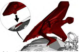
Lower the rear of the windshield assembly and insert the side anchor posts into their sockets. Press down until the posts click into place.
