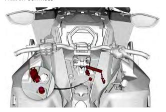
The engine cut-off switch (tether cord) is located on the console.
