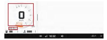
In full gauge view, long press the lower center of the screen to show one the following information. Cycle through the informations with additional long presses.
