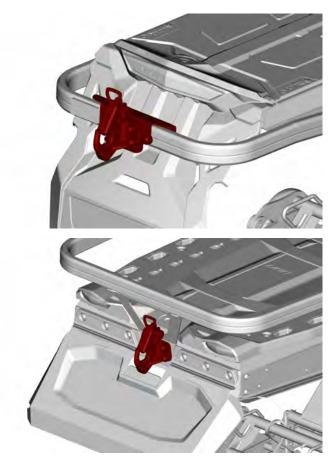
To open the hook, push and turn the handle to retract locking plate.
