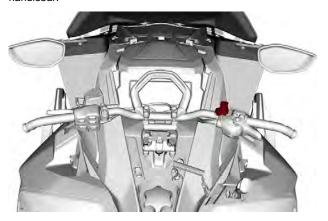
To stop the engine in an emergency, push the switch down in OFF position and simultaneously apply the brake.
