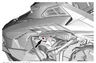
TYPICAL LH SIDE 6. Loosen the air intake duct clamp.
