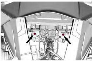
5. Remove the screw and washer that retain the hood trim.
