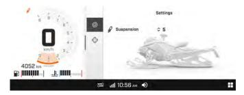
**NOTE**: The display shows the actual suspension setting (a number from 1 to 5, 1 being the softest setting).
