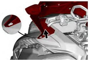
Grasp the windshield assembly under the sides of the windshield support. Lift both sides of the windshield assembly until the side anchor posts are clear of their sockets.
