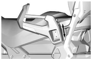
3. Reinstall the screws. Tighten to specification.
