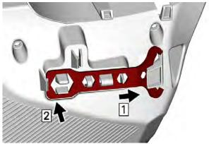
Slide the Pulley expander and headlight adjustment tool short end into hole.
