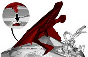
Press the rear corners of the windshield support over the rubber retaining studs.
