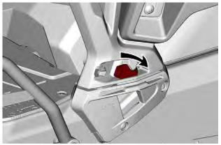
3. Pull the backrest upwards to remove.
