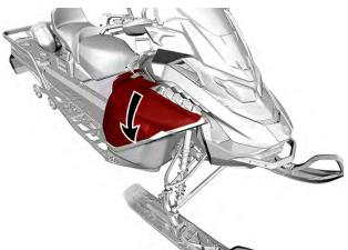
3. Slide the panel hinge off the bottom pan.
