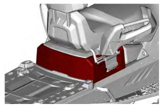
To open, unlatch and tilt passenger seat (if equipped).
