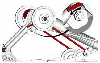
SPRING PRELOAD ADJUSTMENT RH — TYPICAL
