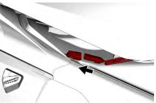
3. Slide the seat forward to engage it with the retaining tabs.
