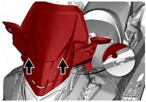
Grasp the windshield support through the vent slot in the front of the assembly. Lift the front anchor post from its socket and remove the windshield assembly.
