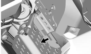
3. Position the rear portion of the belt guard over the retainer and secure it using the retaining pin.
