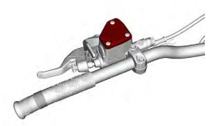
2. Remove the screws retaining the reservoir cap.
