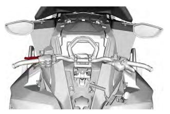
When squeezed, brake is applied. When released, it automatically returns to the resting position. Braking effect is proportional to the pressure applied on the lever and to the type of terrain and its snow coverage.
