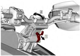
Step 1. Pull lever Step 2. Position handlebar
