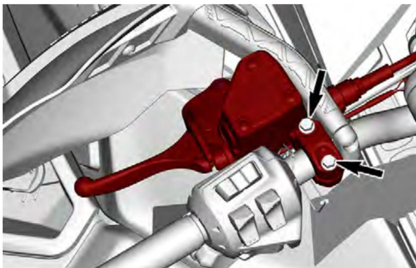
2. Locate the reference mark on the handlebar and respect the distance and rotation limits.
