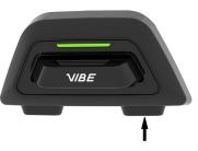
Hold the configuration button for 3 sec to access the configuration menu. You can then go to vehicle pairing by tapping the "up" button twice. Tap the center button to select "vehicle pairing". Then, on your vehicle display, go to Bluetooth settings and select your VIBE UNIVERSAL product in the list of available devices.
