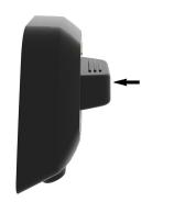
The phone pairing can be activated when the system is off. Press and hold the 2 power on buttons for 3 sec.
