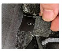
**3.** Position the boom microphone mounting plate on the Velcro.
