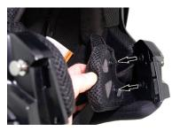
**3**. Position the speakers on the Velcro attachments previously installed while making sure the speaker wires are pointing toward the back of the helmet.
