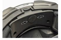
**3.** Position the microphone on the Velcro installed at previous step.
