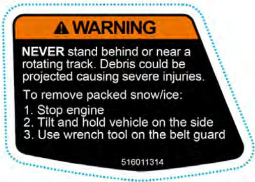
SHREDDER CORE ROTATING TRACK - WARNING LABEL
