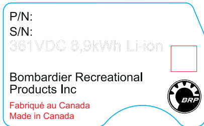
High Voltage Battery Identification Label
