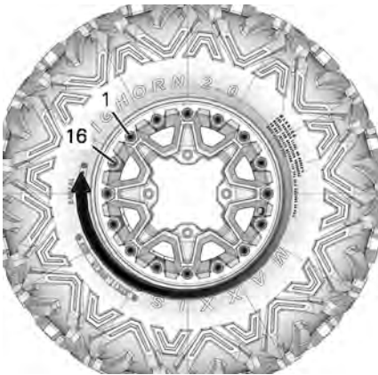
TYPICAL - FINAL TIGHTENING SEQUENCE
