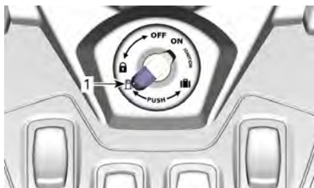
1. Seat opening/fuel cap access
