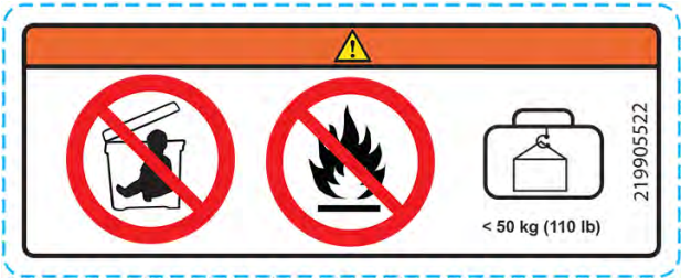
COOLER UTILIZATION - WARNING LABEL
