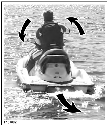
TYPICAL - STEERING DIRECTION REVERSED WHEN BACKING
