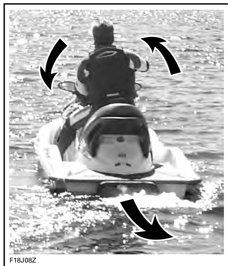
TYPICAL - STEERING DIRECTION REVERSED WHEN BACKING
