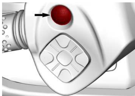
TYPICAL - ENGINE START/STOP BUTTON
