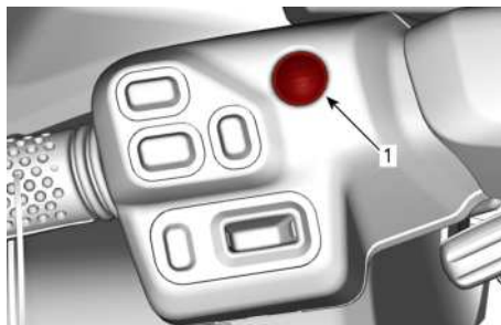
TYPICAL – ENGINE START/STOP BUTTON
