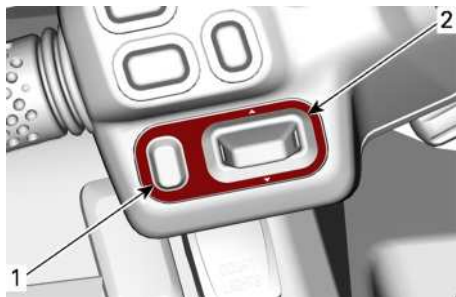
LEFT MULTIFUNCTION SWITCH - LOWER MODULE
