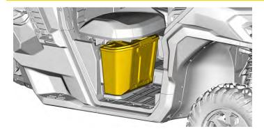
To remove under seat storage box, lift RH passenger seat and remove under seat storage box by pulling it upwards.
