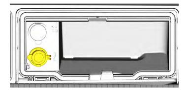
A USB cable extension can be installed from this compartment and used either in the center or side compartments (except HVAC models).
