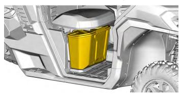
Remove the battery cover by unscrewing the two 1/4 turn fasteners.
