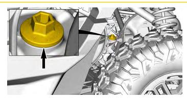
Remove the magnetic gearbox drain plug and discard sealing ring.
