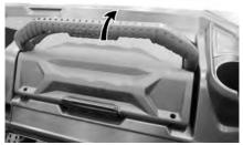
SECURING TOOL BOX IN PLACE
