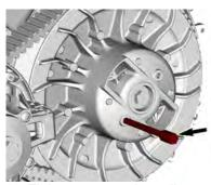
Tighten to open the pulley.
