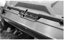
To close the lid, lower it and push the lock upwards.
