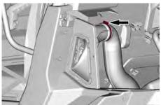
4. Remove filter housing from the vehicle.
