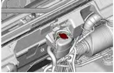
Ensure cooling system is full up to the Max line.
