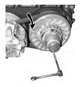
Installing the Drive Belt
