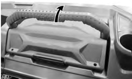
SECURING TOOL BOX IN PLACE
