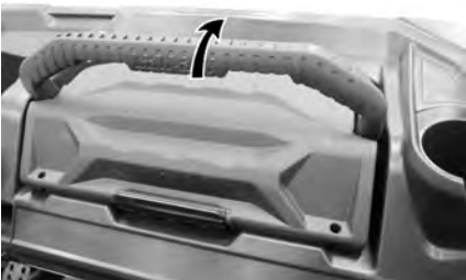
SECURING TOOL BOX IN PLACE
