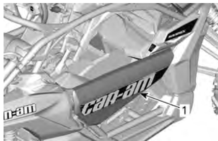
1. Door closed and locked in place
