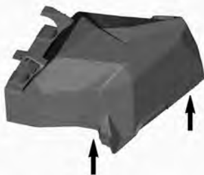
LIFTING REAR OF SERVICE COVER
