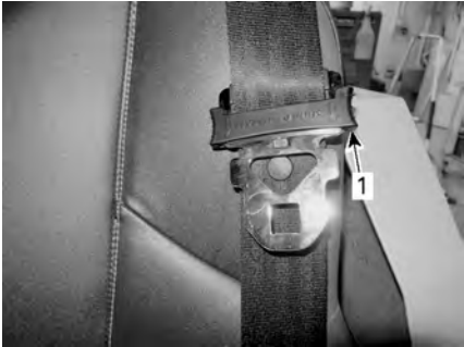
TYPICAL - LOCKED POSITION
