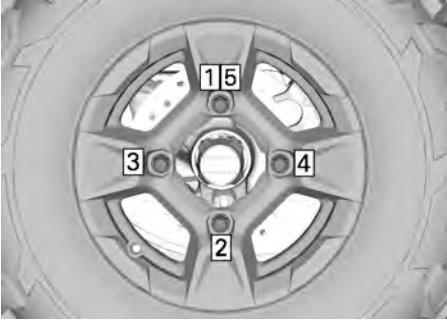
TIGHTENING SEQUENCE
