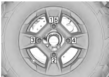
TIGHTENING SEQUENCE
