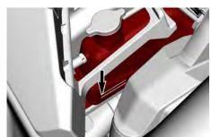
4. Add coolant to the reservoir as necessary. Refer to Cooling System Refilling and Bleeding
