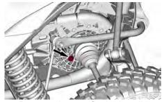
Remove the rear final drive oil level plug and the O-ring.
