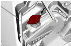
Add coolant until the level reaches the MAX line on the coolant reservoir. Refer to Recommended Engine Coolant. Use a funnel to avoid spillage. Do not overfill.
