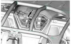
6. Pull towards the front to remove the air intake grille.
