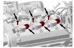
Remove ignition coils with gaskets from spark plug by rotating coil side to side as you pull up.
