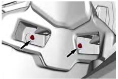
5. Remove the plastic rivet on the top of the air intake grille.
