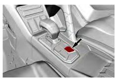
This button engages or disengages the Manual shifting mode.
