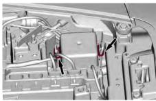
2. Press both tab against the cover and pull it upwards.
