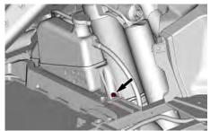
11. On LH side, detach the air filter intake hose from the side baffle.
