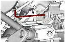
Turn the T30 Torx key toward the driver side (left of the vehicle) until the key stops.
