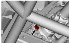
Using a syringe, add the recommended oil. Refer to Recommended Disconnect Unit Oil.
