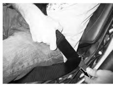
4. To detach the seat belt, push on the red button on the buckle.
