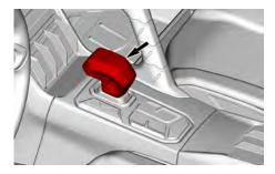
The lever is used to put the transmission into REVERSE or DRIVE (Forward).
