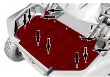
Remove the screws that retain the acoustic baffles to the intercooler support and the chassis. Then remove the baffle from each side of the intercooler.
