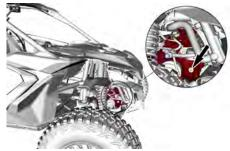
4. Remove the plug and the O-ring.
