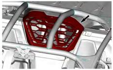
7. Remove the plastic rivets and screws that secure the air intake assembly to the cargo rack. Then remove the air intake assembly.
