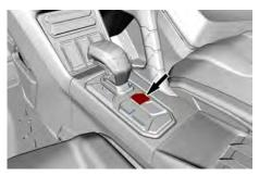
This button allows the low-speed range of the gearbox to be selected.
