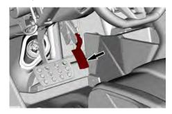
The accelerator pedal controls the vehicle speed and acceleration.
