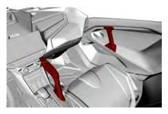
Holding the handholds helps the passenger brace against the movement of the vehicle and helps keep hands and body inside the cockpit in the event of a rollover.
