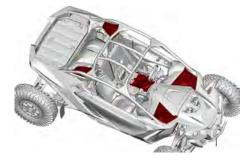
The audio system is composed of four speakers and one subwoofer enclosures.
