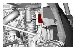
Remove the Oetiker clamps that secure the inlet and outlet hoses to the pre-filter.
