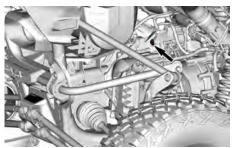
Insert the T30 Torx key, (located in the vehicle tool kit) in the end of the transmission shifter shaft through the access hole.
