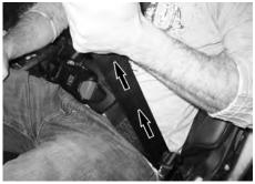
To loosen the seat belt, hold the lap belt with one hand and pull the red strap outwards.
