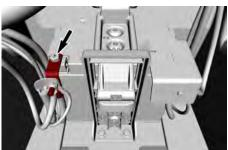
Remove the two hex head screws and flat washers that secure the battery holder to the bottom of the battery compartment.
