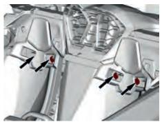
Remove the four screws, two behind each seat, securing the intercooler support to the rear central partition.
