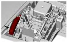
Begin by connecting one end of the RED jumper lead to the positive (+) post of the discharged battery.
