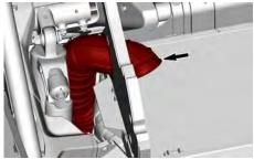
Remove the screws from the intercooler support. Then remove the intercooler.
