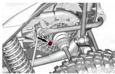
From the underneath the vehicle, through the skid plate hole, clean the area around the magnetic drain plug.
