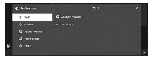
If no Wi-Fi network is available near the vehicle, you can share your smartphone cellular network by hotspot. Just note cellular data fees may apply. The 10.25" touchscreen display will only connect to a secured network.
