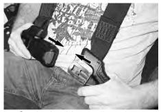
On both sides, adjust the seat belt tightly against your body by pulling the excess of the lap belt towards the inside. The buckle must be centered at the waistline (as low as possible).
