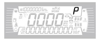
This display shows gear position of gearbox:
