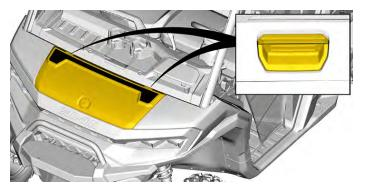
3. Locate the brake fluid reservoirs.
