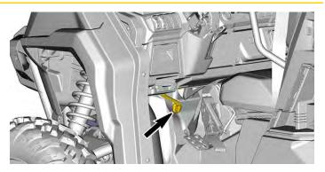
The brake holding mechanism function is to maintain brakes to all wheels while shift lever is set to Park.
