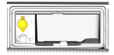
Remove the protective cap to use. Always reinstall it after use to protect against intrusion.
