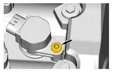
6. Pull and twist the ignition coils both sides to remove them with their gaskets.
