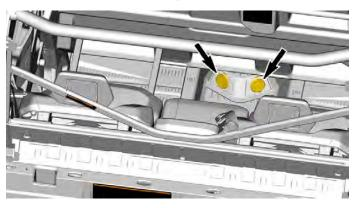
To allow or stop the airflow, open or close the outlet.
