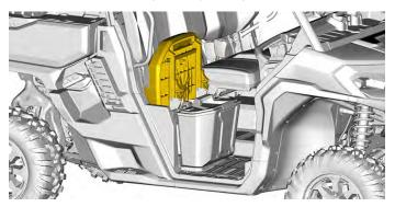
When reinstalling the storage box, make sure to align it properly with the floor emboss so it fits properly under the seat.
