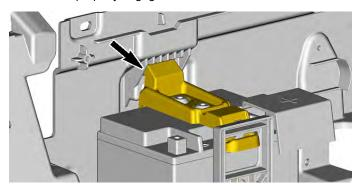
3. Install the battery holder screws.
