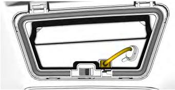
The USB cable can be removed from this compartment and used either in the side compartment (except HVAC models) or in the smartphone holder.
