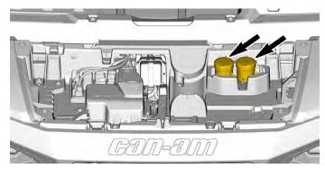
Using the marks on the brake fluid reservoirs, check the fluid level. The proper level should be between the MIN and MAX lines.
