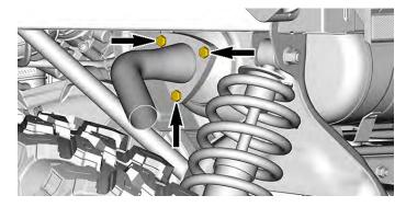
2. Remove the exhaust tail pipe and the spark arrester.
