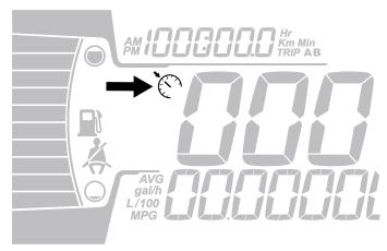
Activating utility speed limiter mode of operation only limits the maximum speed available when depressing the throttle.
