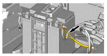
The other one is located under the front hood, attached to the POS (+) post.
