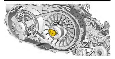
Install the puller/locking tool in the driven pulley adaptor threaded hole. Tighten the puller/locking tool to completely open the pulley.
