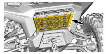
Visually, inspect the radiator fins. They must be clean, free of mud, dirt, leaves or any other deposit that would prevent air from passing freely trough the radiator. 5. Using a garden hose, rinse the radiator fins.
