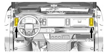
To adjust or close the airflow direction, move the tab.
