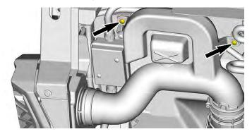
3. Disconnect the air intake side of the resonator. Set the resonator aside.
