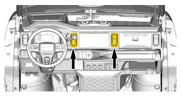
To adjust or close the airflow direction, move the tab.
