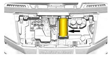
2. Slide rearward, lift then slide forward the filter to remove it.
