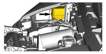
3. Ensure the cooling system is full up to the MAX line.
