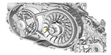
To remove belt, slip the belt over the top edge of fixed sheave.
