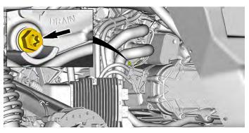
12. After draining, squeeze the coolant hose just above the drain plug a few times to drain more coolant.
