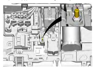
5. Then connect the other end of the RED jumper lead to the positive (+) post of the booster vehicle's battery.
