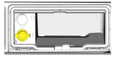
A USB cable extension can be installed from this compartment and used either in the center or side compartments (except HVAC models).
