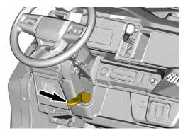
2. Move steering wheel to the desired position.
