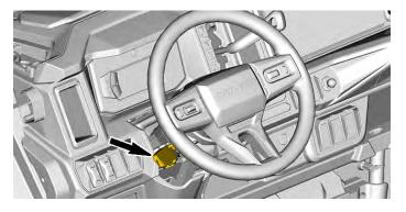
After seating, just lower to clip back in place. The steering wheel returns to the adjusted height before by the operator.
