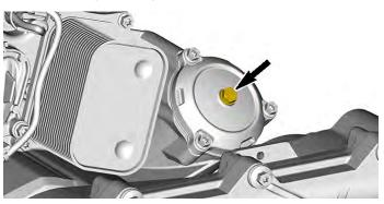
5. Empty the oil filter housing by activating the vacuum/pressure pump in pressure mode 10 to 15 times.
