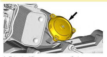
6. Tighten the oil filter cover screws to specification.
