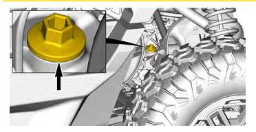
6. Remove the magnetic gearbox drain plug and discard sealing ring.
