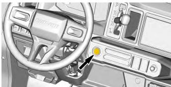
With the D.E.S.S. key inserted, press and hold the Engine Start/ Stop button to start the engine.
