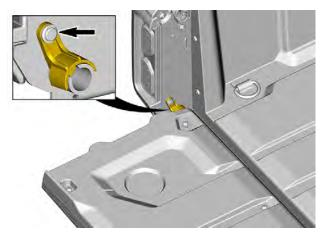
3. Gently pry the spring clip past the screw head on each side.
