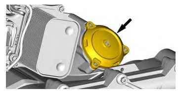
8. Remove and discard the engine oil filter.
