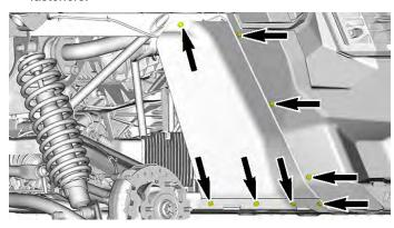
9. Remove the rear skid plate by removing the following fasteners on both sides.
