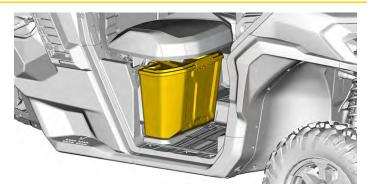
To remove under seat storage box, lift RH passenger seat and remove under seat storage box by pulling it upwards.
