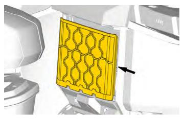
3. Install a new air filter and the grille.
