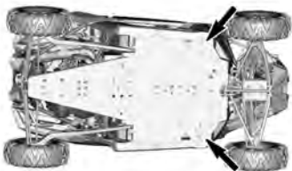
JACK STAND POSITIONS - FRONT OF VEHICLE
