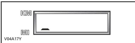
However, if the speedometer shows another number than **511---**, release and repress the button. The number should be change for **511---**. Hold the button to change the unit until the normal display comes back.
