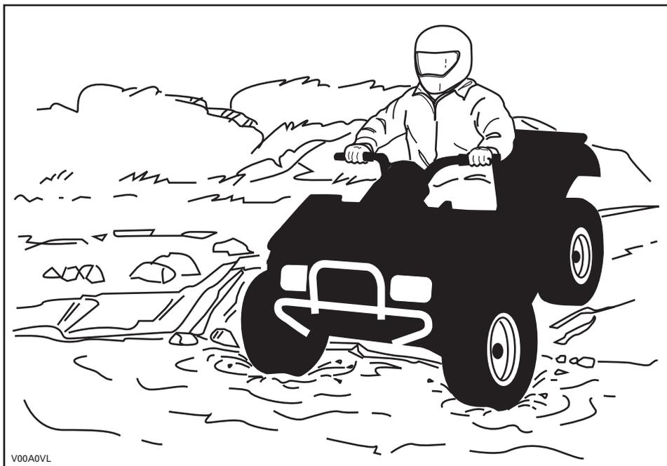
Water will affect the braking ability of your ATV. Make sure you dry the brakes by applying them several times after the ATV leaves the water.
