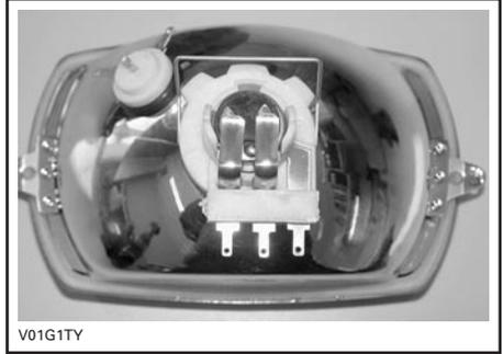
Remove the socket snap. Open the both side of socket snap.
