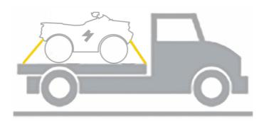
Transport vehicle on a flatbed truck or comparable transport vehicle using suitable tiedowns. The vehicle needs to be secured onto the platform facing forward.
