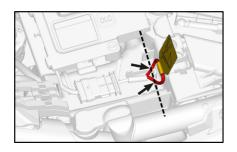
1. Double cut the loop adjacent to the label to prevent wires contact.
