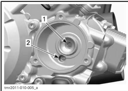
1. Outlet bore to the engine oil providing system
