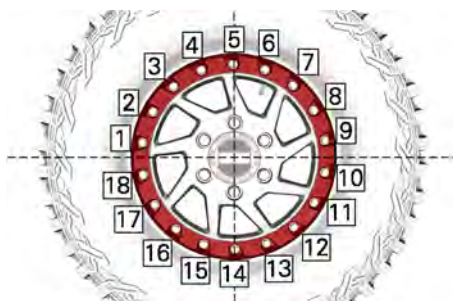
TYPICAL - FINAL TIGHTENING SEQUENCE
