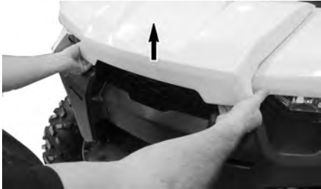
LIFTING FRONT SERVICE COVER EDGE.
