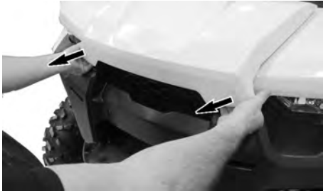
PULLING ON FRONT SERVICE COVER EDGE.
