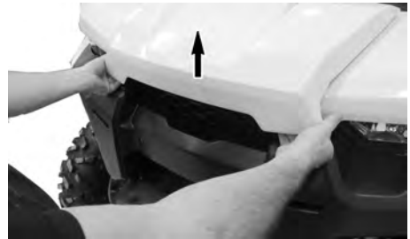
LIFTING FRONT SERVICE COVER EDGE.
