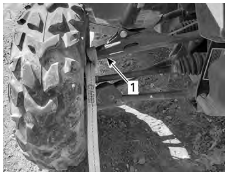
1. Front upper suspension arm
