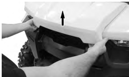
LIFTING FRONT SERVICE COVER EDGE.
