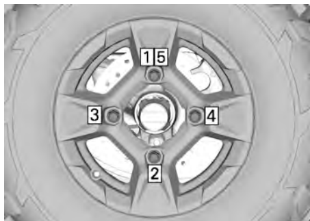
TIGHTENING SEQUENCE
