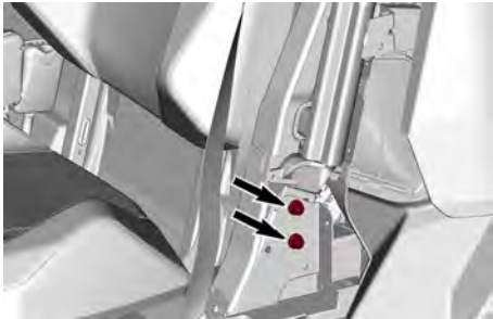
REAR CAGE FASTENERS
