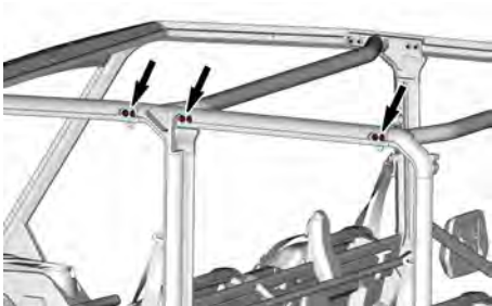
TOP CAGE FASTENERS
