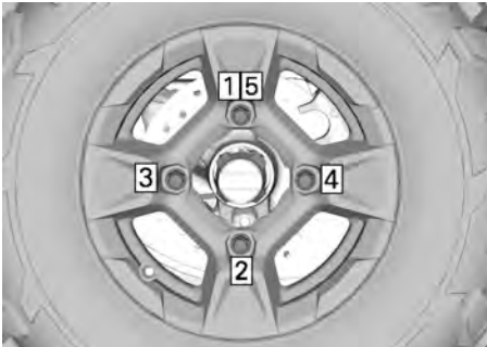
TIGHTENING SEQUENCE
