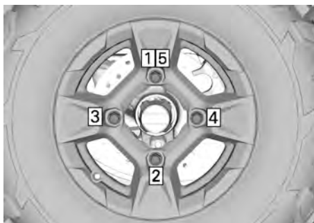
TIGHTENING SEQUENCE
