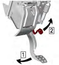
Step 1. Apply and hold brake pedal Step 2. Lift lever
