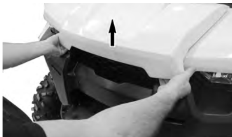
LIFTING FRONT SERVICE COVER EDGE.
