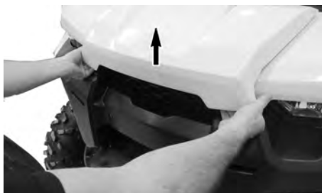
LIFTING FRONT SERVICE COVER EDGE.
