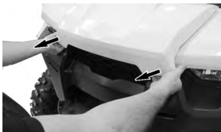
PULLING ON FRONT SERVICE COVER EDGE.
