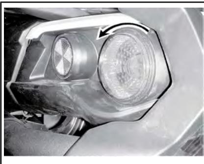
**RUOTARE IL FANALINO IN SENSO ANTIORARIO PER RIMUOVERLO**
