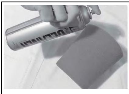
*TYPISCH - SCHAUMSTOFFFILTERELEMENT BESPRÜHEN*
