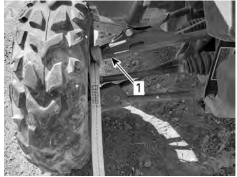
1. Front upper suspension arm
